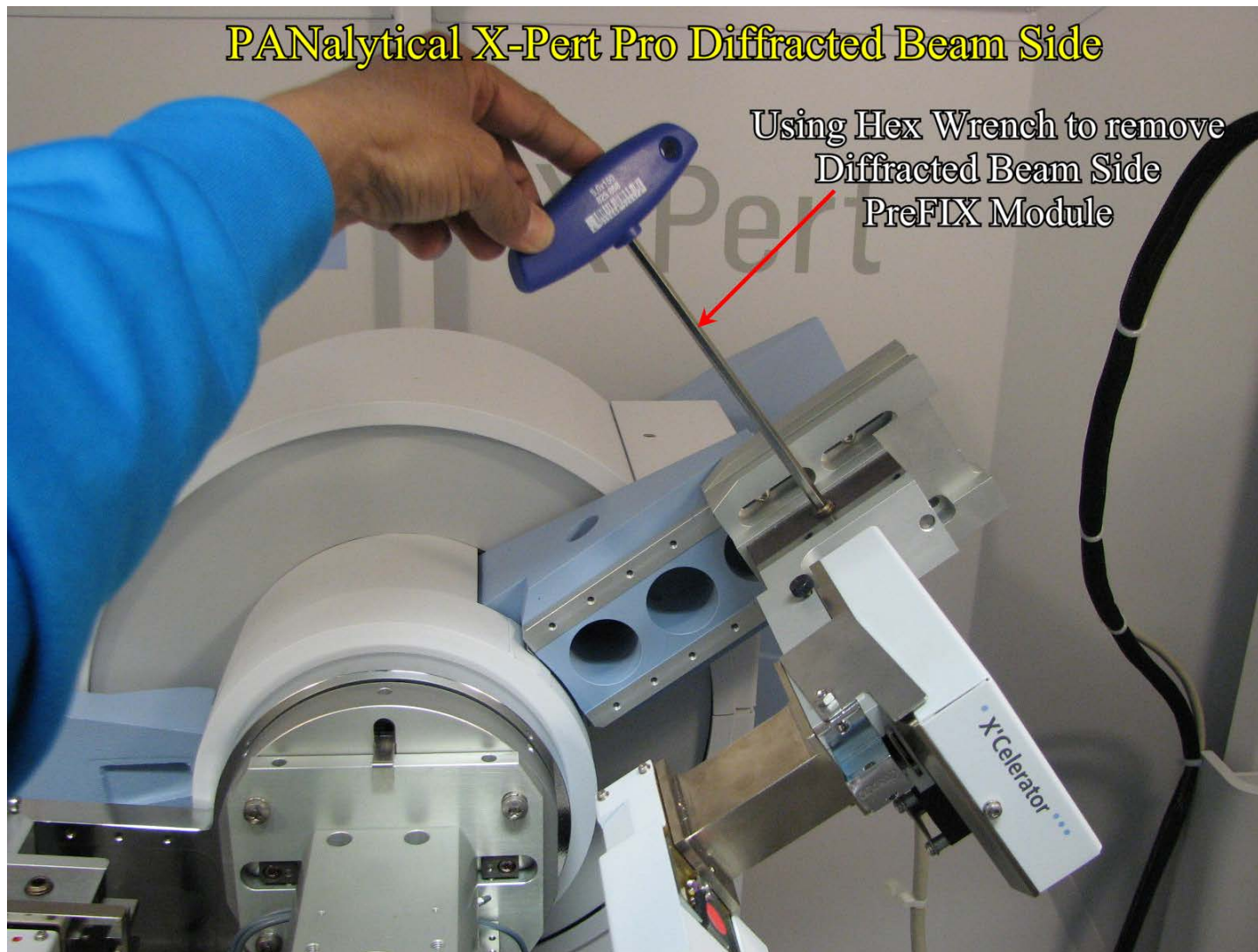
PANalytical X-Pert Pro Powder Instrument at FSU CSL 1011 using hex wrench to remove diffracted beam side PreFIX module
