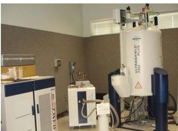
700 MHz AVIII with Cryo-probe
